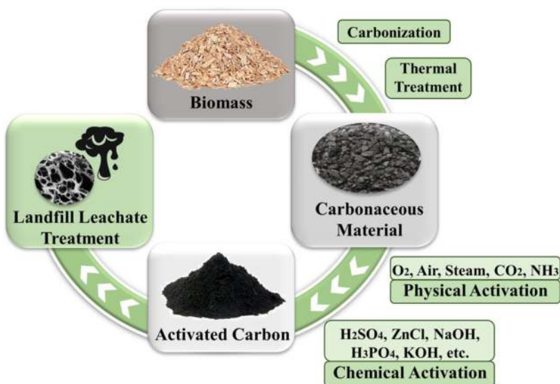
Figure 10.1 Schematic diagram of the activation techniques for AC production from biomass.
