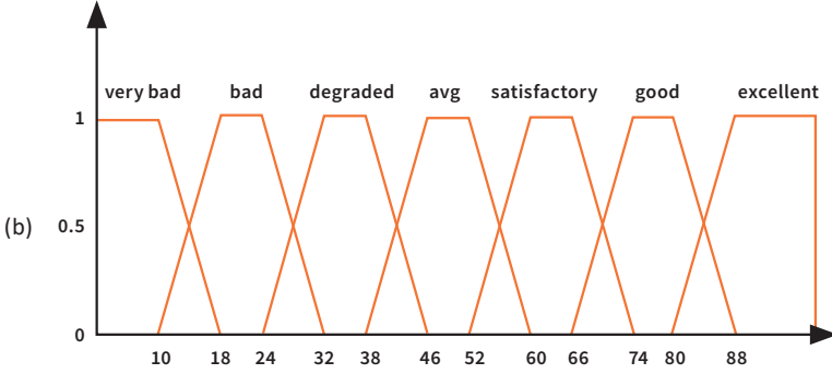
Figure 6. (a) Quality and (b) QA score membership functions. Source: Reprinted from Kuwelkar and Virani (2021b), used with permission.
