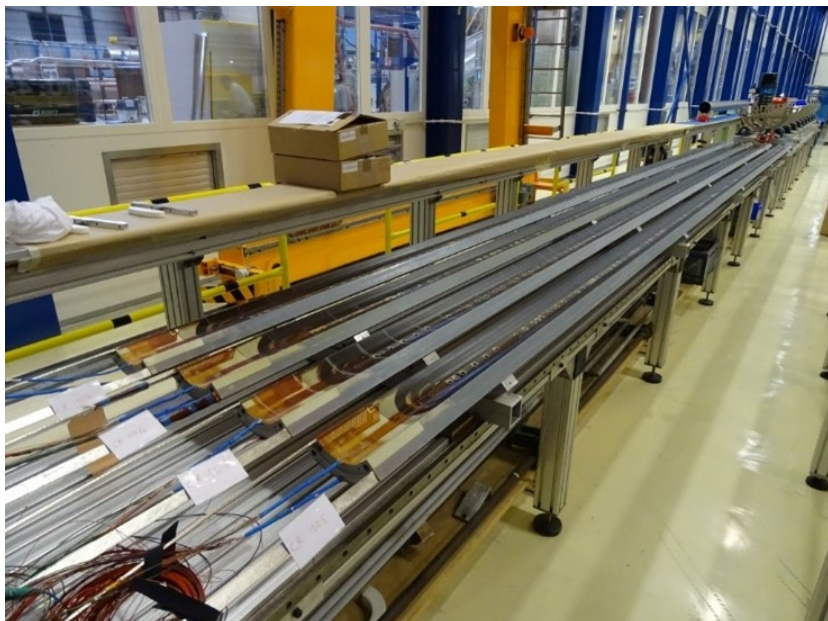
Fig. 13. MQXF coils manufactured at CERN.
