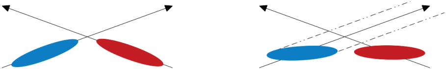
Fig. 1. Bunches colliding with a crossing angle without crab crossing (left); with the crab crossing (right).
