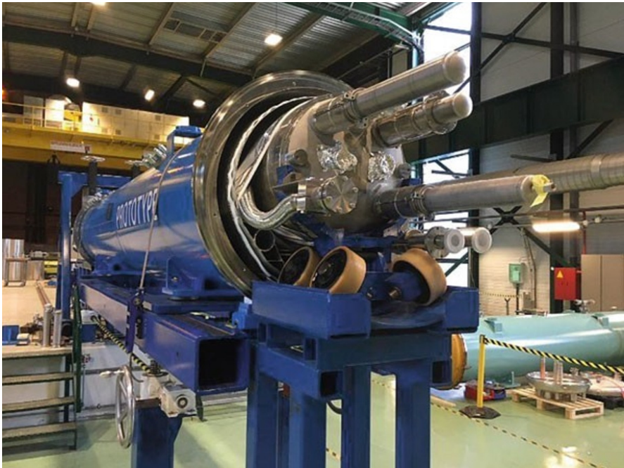
Fig. 10. The first 5.5 m long 11 T MBH dipole prototype in its cryostat at CERN ready to be transported to the test bench.
