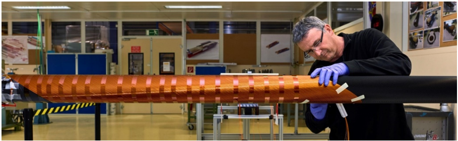
Fig. 10. Winding the first CCT prototype at CERN.
