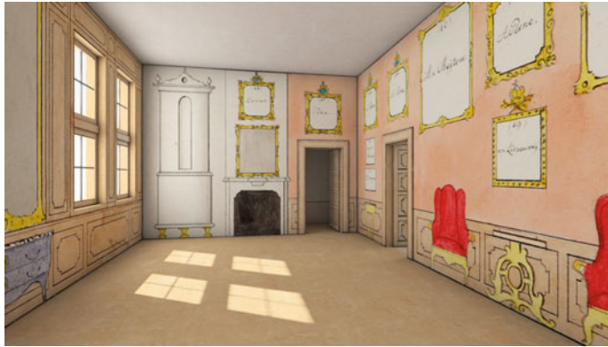
Fig. 7.8 Projection of the original sources on the 3D model, Art gallery castle Schwerin (Image: Architectura Virtualis, Darmstadt 2018)
