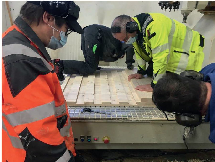
Figure 9. Manufacture of dovetail massive wood board element at Vocational College Lapland (Ammattiopisto Lappia), Kemi, Finland (photo by Hüseyin Emre Ilgin).
