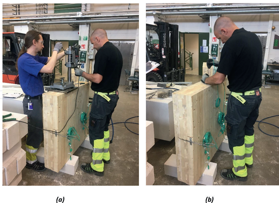
Figure 10. Preparation of dovetail specimens for fire resistance test at Tampere University Fire Laboratory, Tampere, Finland. (a) Drilling and (b) thermocouple insertion (photos by Hüseyin Emre Ilgin).
