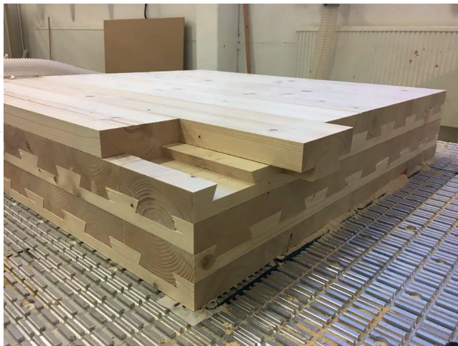
Figure 5. Test specimen of adhesive- and metal fastener-free dovetail wood board element (photo by Hüseyin Emre Ilgın).
