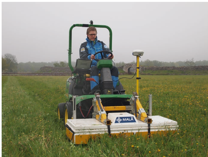
Fig. 4 Collecting of GPR data at the fortress of Gråborg. (Photo: Magnus Larson)
