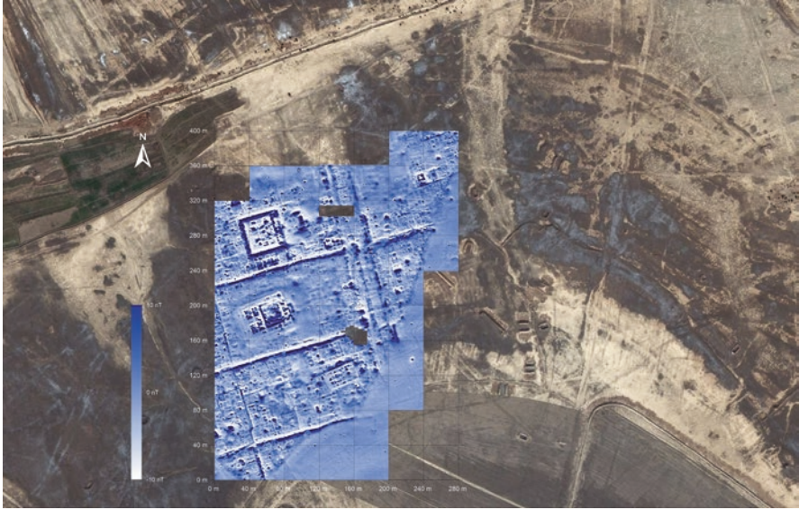
Fig. 13 Charax-Spasinou. Magnetogram fused by a satellite Image (Google-Earth) Scintrex SM 4G-Special Caesium magnetometer in a duo-sensor and total field configuration (grid-size of magnetograms 40 × 40 m)
