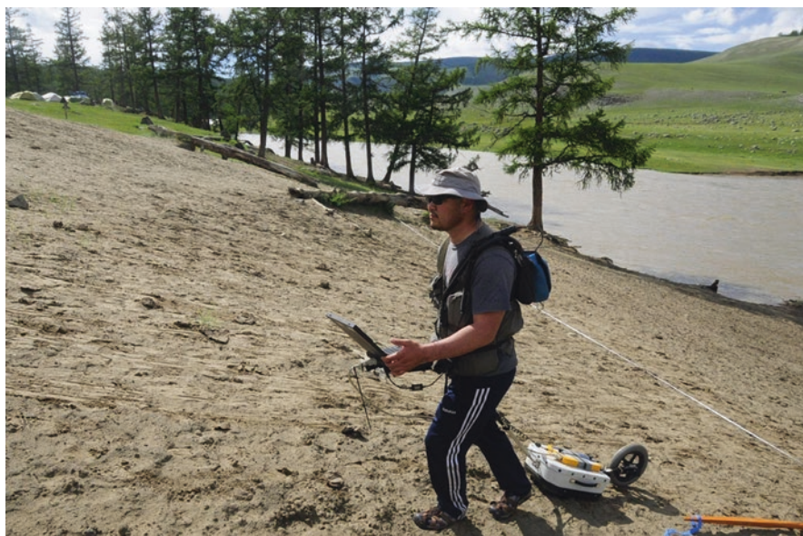
Fig. 4 GPR being used to map the stratigraphy of the Soyo site in Northern Mongolia by Dr. Bayarsaikhan Jamsranjav, as discussed in Vella (2018)
