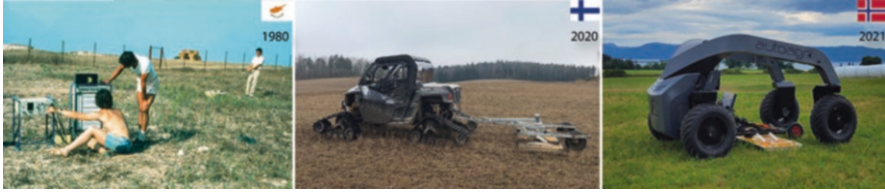
Fig. 1 Evolution of (ground-based) geophysical instrumentation, taking ground-penetrating radar (GPR) systems as an example. From left to right: (1) One of the first GPR surveys in archaeology carried out at the Bronze Age site of Dromolaxia-Vyzakia, near Hala Sultan Tekke mosque in Larnaca, Cyprus (Courtesy Peter M. Fischer, University of Gothenburg, Sweden); (2) First Finnish archaeological GPR survey using a multi-channel system at Iron Age sites of the Karjaa Lepinjärvi area (Courtesy Arne A. Starnes, NTNU, Norway); (3) First autonomous archaeo-geophysical survey at the Viking age burial site of Rygg in Frosta, Trøndelag, Norway
