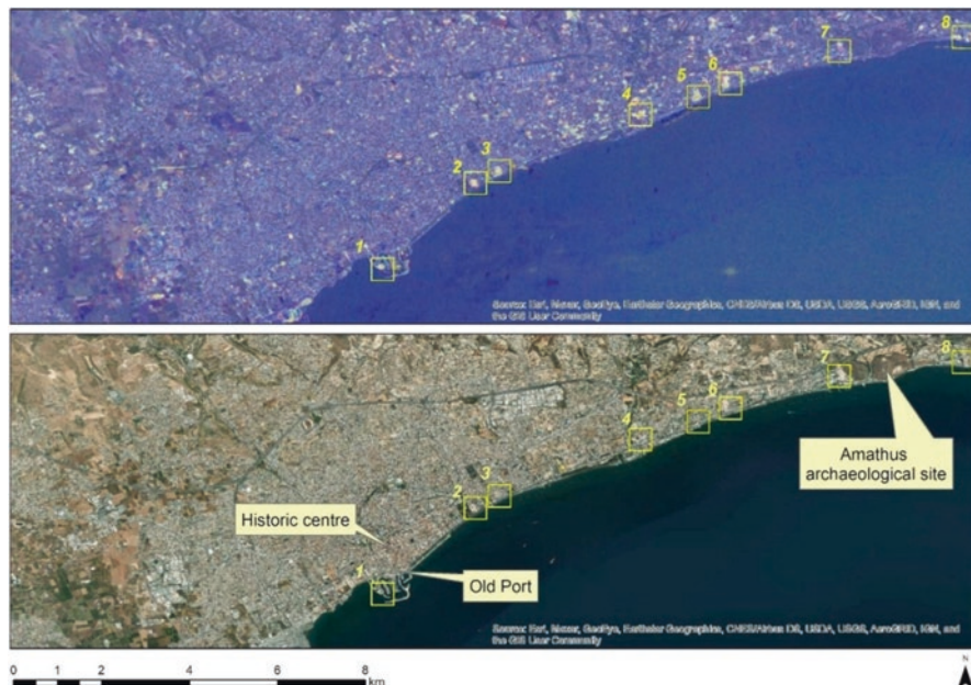
Fig. 10 Top: Radar polarisation visualisation change detection during the period 2015–2020 over Limassol city. Bright colours indicate areas of changes during this period. Bottom: The same are using as a background a high-resolution satellite image. (Source: ArcGIS Basemap)
