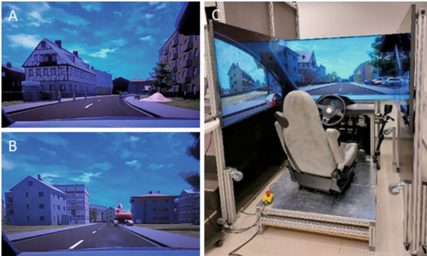
Fig. 2 The cooperative scenarios of the simulator study, two-sided bottleneck (A) and one-sided bottleneck (B), which were implemented in DLR's coupled simulator AIM MoSAIC (C)
