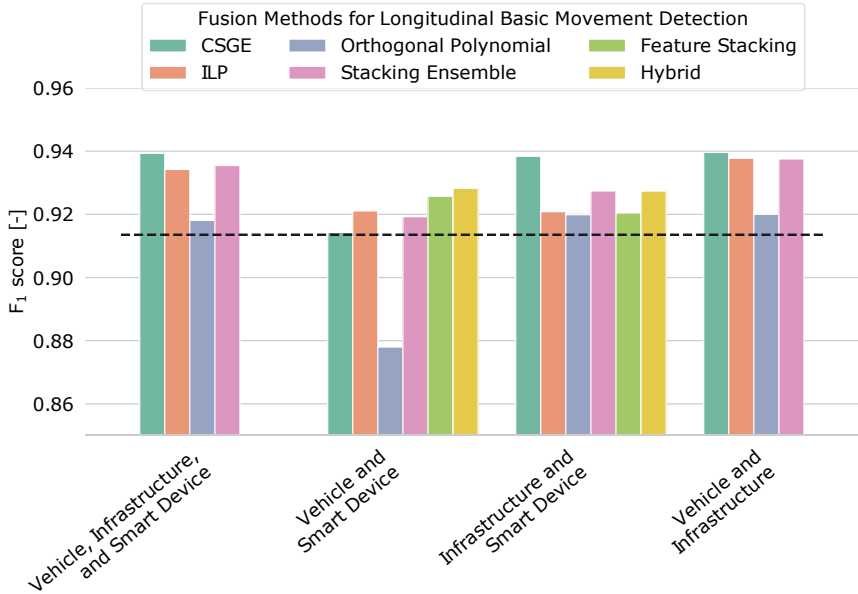
Fig. 21 Micro average F_1 score for cooperative longitudinal basic movement detection. Results of cooperative longitudinal basic movement detection for different agent configurations. The colored bars represent different fusion types. The baseline, i.e., the ego vehicle only, is given by the black, dashed line [7]
