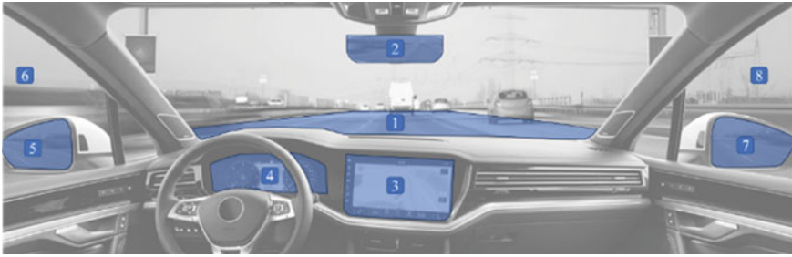
Fig. 4 AOIs according to the numbering of ISO 15007:2020 (adapted from Herzberger [23])
