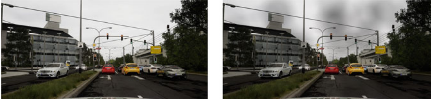
Fig. 8 Original image generated with CARLA on the left and image with dust on the right with 60 simulated particles and a distance of 50 mm distance to sensor
