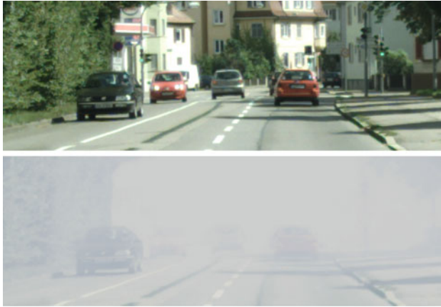
Fig. 10 The upper image is from the Cityscapes data set [14], the lower image shows the image with our fog simulation applied. Image from [7]
