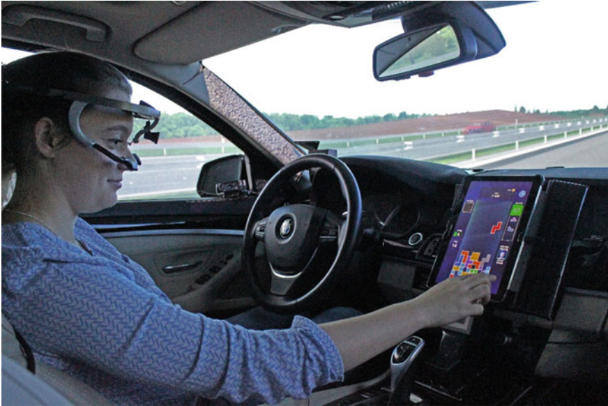
Fig. 3 In-vehicle study setup in the static driving simulator of the Institute of Automotive Engineering (ika) at RWTH Aachen University
