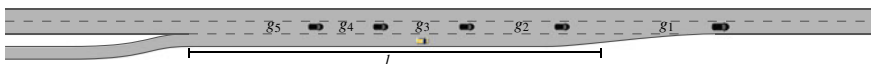
Fig. 11 Overview of the map and gap identifiers; gap g_5 has no longitudinal lower bound in this case, adapted from [26]
