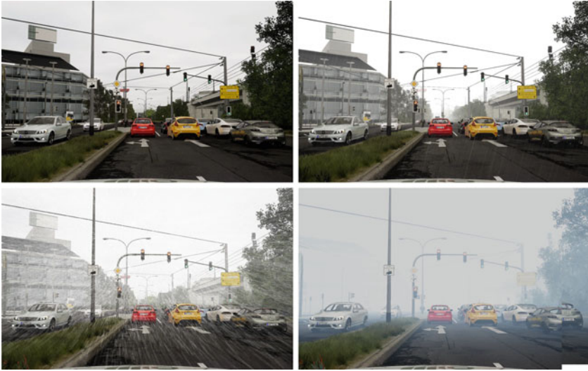
Fig. 2 Example image generated with CARLA simulator [19] with the proposed weather augmentations (original, rain, snow, fog) from Sect. 2
