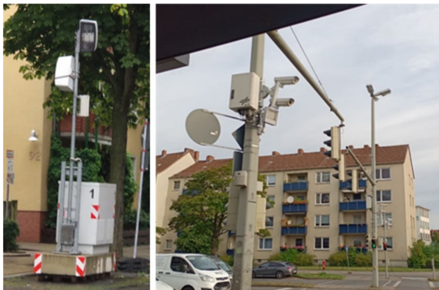
Fig. 1 DLR's application platform for intelligent mobility (AIM) research junction (right) and mobile installations (left)
