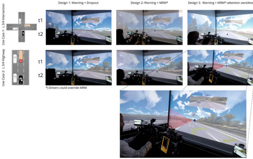
Fig. 8 Simulator study of confidence horizon designs in two use cases ( N = 20 , Snapshots from the gaze scene video, blue dot represents drivers gaze)
