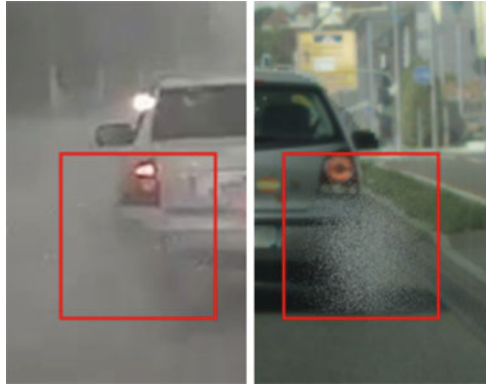
Fig. 7 Qualitative comparison of real spray (taken from the realrain data set [112]) on the left, and our simulated spray on the right. Because of the lack of clean spray data sets, we can only compare the occlusion of the lower end of the vehicle. Here, we can observe similar behavior: parts of the wheel are not visible, as well as part of the rear end and parts of the rear lights. The spray color blends in with the background and the color of the street; it reaches the same height as the real spray. Image from [113]
