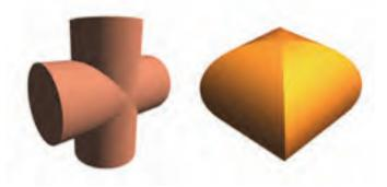
Fig. 17. Intersection of two cylinders
