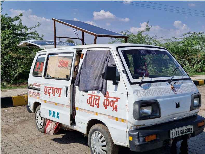
Figure 7.4 Solar PV on an emissions testing van off the highway in Jaipur. © The author
