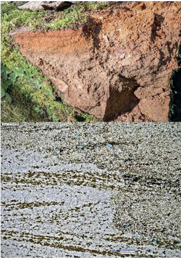
Figure 2.6: Top: Weathered stone in stream bed at Shawk, with fresh stone at the bottom and darker bands of weathered stone toward the top. Bottom: thin section across weathering profile of sandstone from Hartley Bay (HB002) with fresh stone bottom left and the darker more iron rich weathered stone across the top of the image and down the right-hand side.
