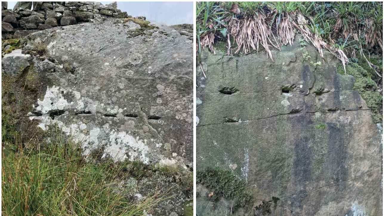
Figure 4.10: Left image – line of wedge holes at Queen's Crag quarry, Northumberland ; right image – wedge holes with visible toolmarks at Comb Crag quarry, Cumbria .
