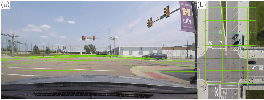
Fig. 2. Sample output grid of the modified YOLOv5 network mapped on the (a) roadside and the (b) top view. The (a) roadside view is the input of the network.
