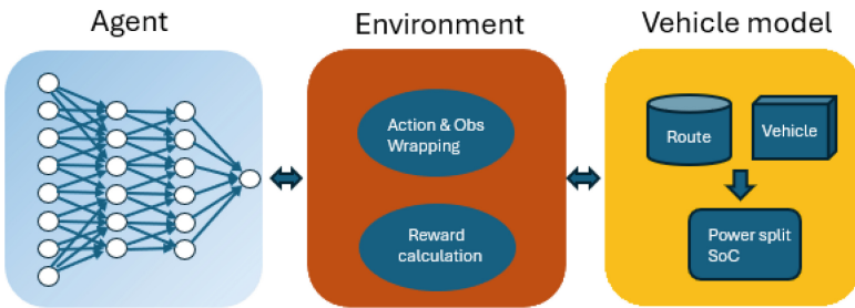
Fig. 1. Training architecture. The agent forms a deep reinforcement learning algorithm, which takes observations from the vehicle model as inputs and outputs the action. The environment sends a step/reset command along with the action to the vehicle model. The vehicle model integrates the next step's power requirement and the current power split observations based on the action and sends it back to the environment. The environment checks for termination/truncation of the episode based on the observations from the vehicle model. The environment then calculates the reward, which is used to update the agent's network. Additionally, the environment normalizes the observations and feeds them back into the network.
