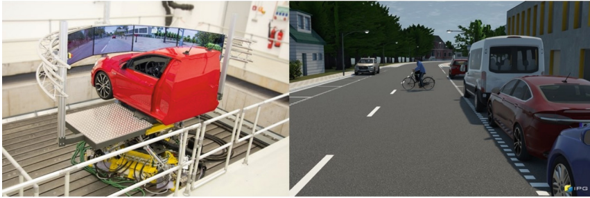
Fig. 1. Dynamic Vehicle Road Simulator (DVRS) of the Institute of Automotive Engineering (left) and scenario (1) with a crossing cyclist (right)
