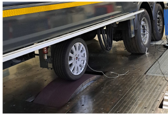
Fig. 3. MoLAS semi-trailer on the RuotaVia drum.
