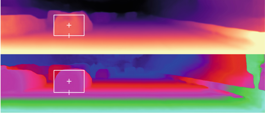
Fig. 1. Depth map samples for image number 150 of split 20 in the Kitti Tracking dataset [4]. Above the depth map of the Monodepth2 inference is shown, below the results of the 2D-MSNet. A ground truth bounding box is highlighted with both reference points (center: Monodepth2 and 2D-MSNet, center bottom: IPM). In both color variations, darker colors represent distance. Lighter colors emphasize proximity.
