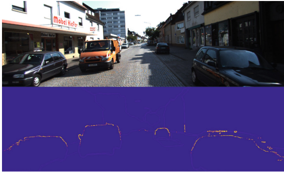
Fig. 2. Sample result of extracted key points of occluded areas. The top image is showing the original RGB image and the bottom image is showing the extracted key points of occluded areas made by the vehicles and building seen in the RGB image.
