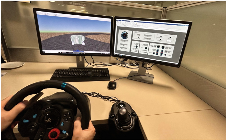
Fig. 4. Steering Maneuver from DIL Simulation
