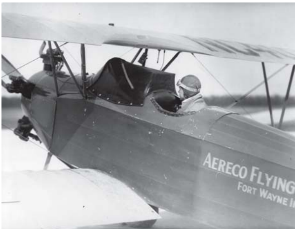
A blind-flying hood was used in flight training to teach pilots how to rely on their cockpit instruments for guidance. (Author's collection)
