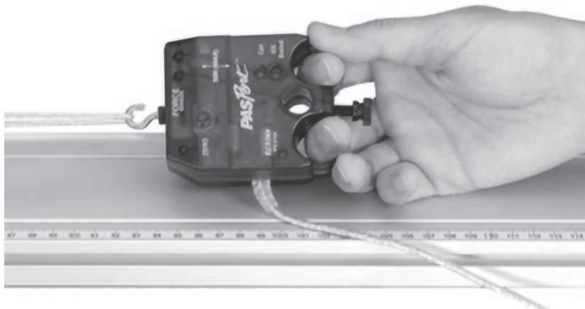
FIGURE C.7 String connected to the force sensor.
