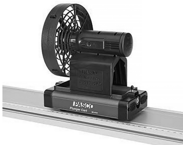
FIGURE C.4 Cart with a fan on the track.
