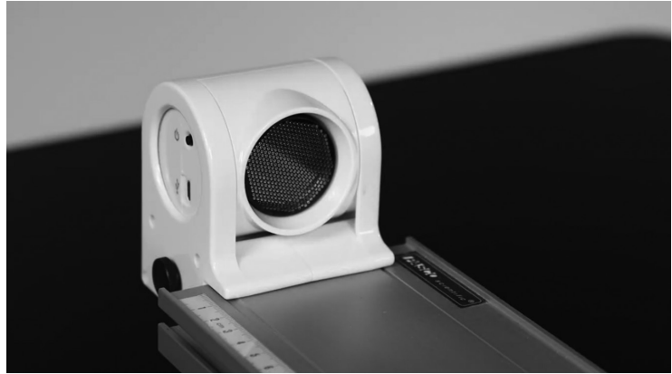
FIGURE C.2 Dynamic cart track with motion sensor.
