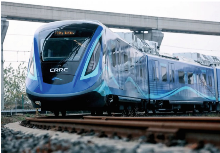
Fig. 3.9 CRRC 160 km/hour zero emission hydrogen train in February 2023. Source: (Hackaday 2023) Image copyright CRRC. All rights reserved
