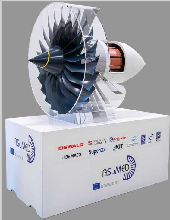
Fig. 5.3 Mock-up of a fully superconducting liquid hydrogen cooled 1 MW motor presented at the 2019 Hannover Fair. Source (Ball 2022), Image rights: IOP Publishing via STM Permissions Guidelines
