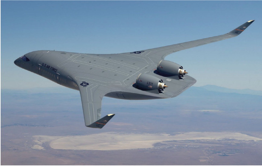
Fig. 3.10 Rendering of a US Air Force blended wing body aircraft concept to be progressed by JetZero pioneers in blended wing body design (U.S. Air Force 2023)
