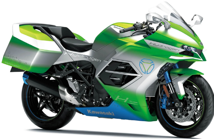
Fig. 3.8 Kawasaki HySE hydrogen fuelled ICE motorcycle concept. Source: (Williams 2022) Image copyright Kawasaki Motors, Ltd. All rights reserved
