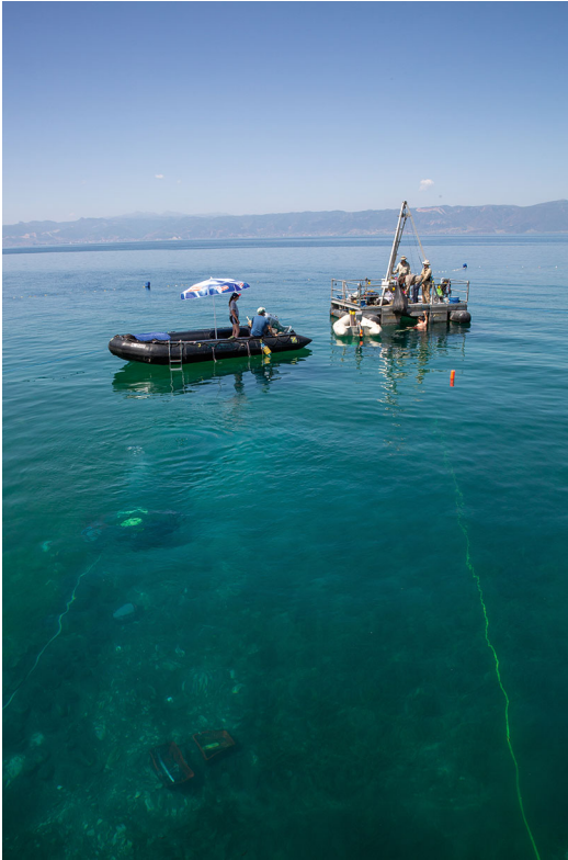
Fig. 6.4 Ploča Mičov Grad. Drill coring with the UWITEC platform and simultaneous pile field documentation and sampling under water (M. Hostettler, EXPLO/UBern)
