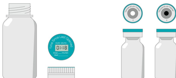
Fig. 19.3 Example of bottle lid indicating the time elapsed since the last opening (on the left); Bottle with marker that changes its color if the product has been exposed to a temperature outside the range of acceptability (on the right)
