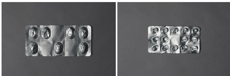
Fig. 16.19 Here is an example of aluminium-aluminium blister deformation making a challenging use due to interference with the secondary packaging and the leaflet when reinserting the blister after use
