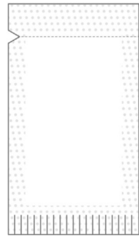
Fig. 22.12 Example of a micro-design to indicate to the user the 'tear-off' opening point of the package. The point should be placed on the left to accommodate the gestures that are normally made by the user
