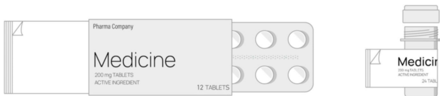
Fig. 19.1 A blister that slides, presenting a “book leaflet” from the opposite side (on the left side) and bottle with unrollable leaflet (on the right). With these types of packaging, the patient has the whole package leaflet available at every medicine intake
