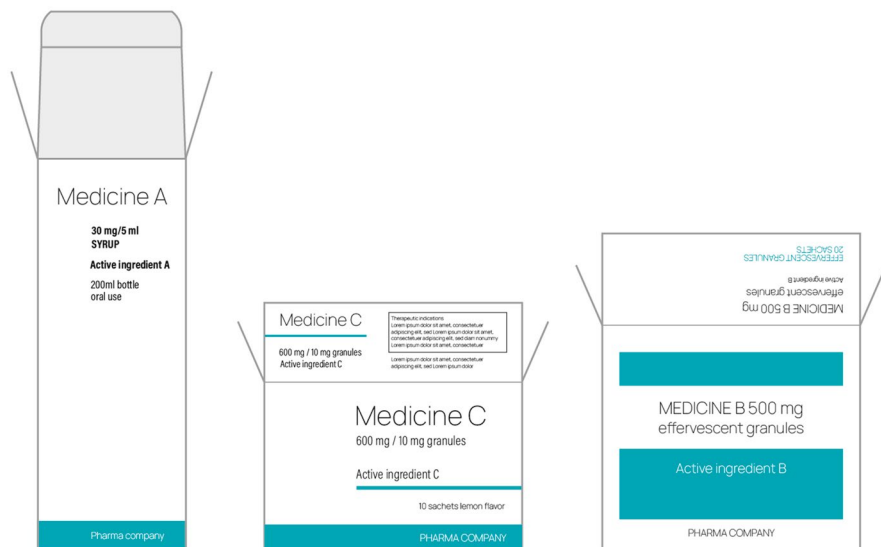
Fig. 17.16 On the left the syrup package with the correct opening of the top. In the centre packaging containing powder in sachets, with the top opening from the back towards the front. In doing so, the user turns the packet over, thus losing information about the pharma they are taking. The third picture even shows the same situation as the pack in the centre, but on opening, the cover graphic appears ‘upside down’
