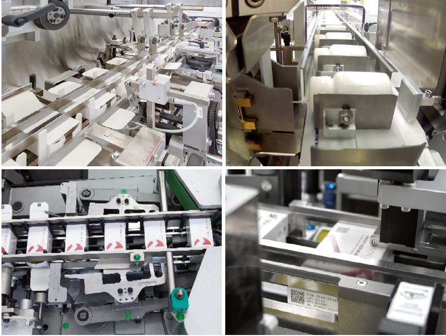
Fig. 5.1 From top-left to bottom-right: packaging opening, filling, closing and stamping. (Source: the author)
