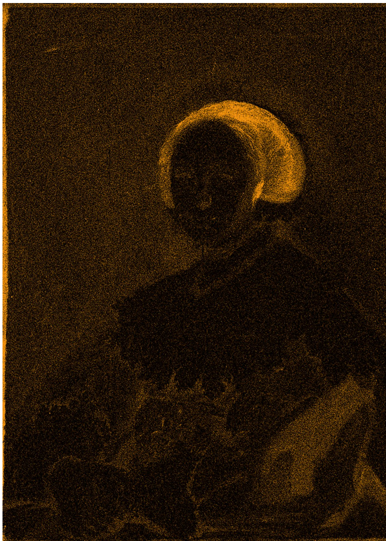
Fig. 3.9 MA-XRF scan of Fig. 3.1, showing the element manganese (Mn)
