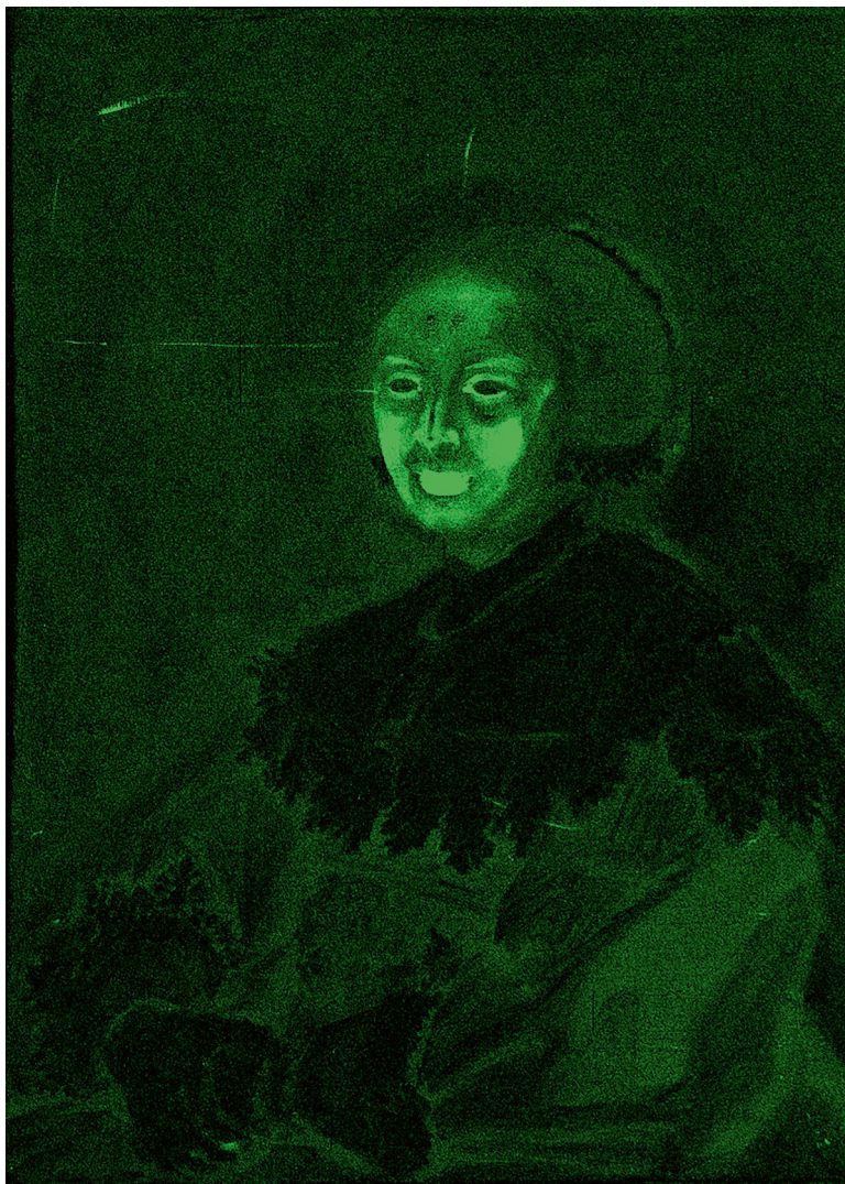
Fig. 3.15 MA-XRF scan of Fig. 3.1, showing the element mercury (Hg)
