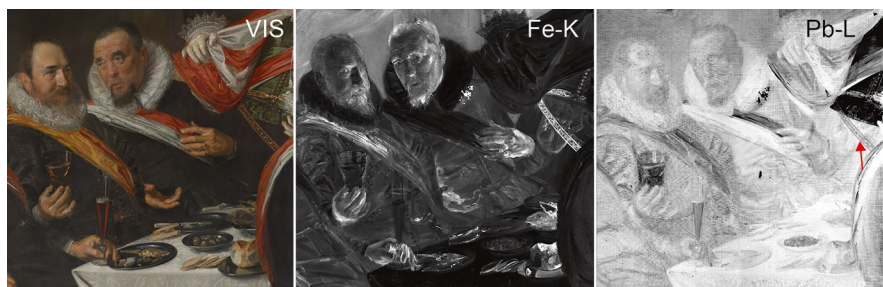
Detail of Fig. 6.1: visible light image, iron (Fe-K) map and lead (Pb-L) map, in ‘sync mode’ ( sn.pub/xtdeqv )
