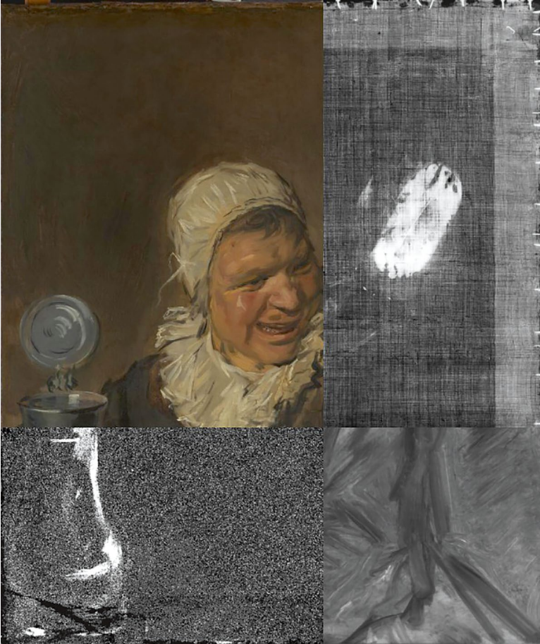
Fig. 7.4 Four different imaging modalities of the Malle Babbe (1632–1635, Staatliche Museen zu Berlin, Gemäldegalerie) are viewed simultaneously with the ‘curtain mode’ of the Curtain Viewer. Clockwise from top left: visible light photography, x-radiography, infrared reflectography, Cu-K MA-XRF map
