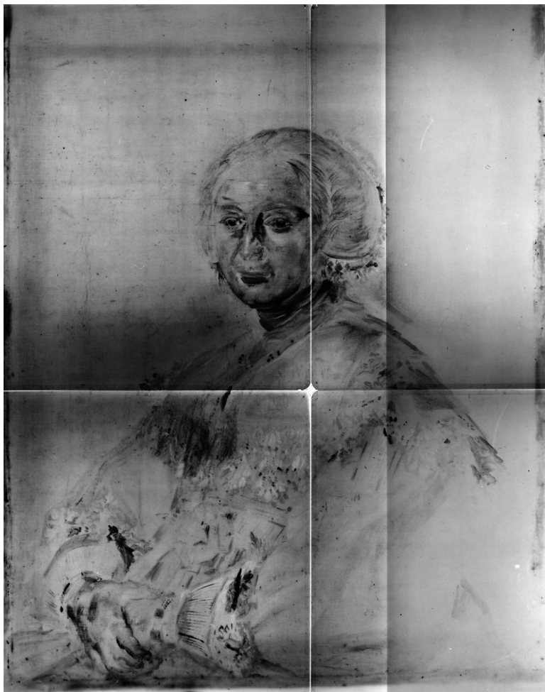
Fig. 3.13 Neutron-autoradiograph of Fig. 3.1 (second recording)
