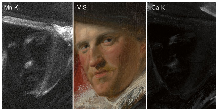
Detail of Fig. 6.1: manganese (Mn-K) map, visible light image, calcium (Ca-K) map, in 'sync mode' ( sn.pub/p9nhja )
