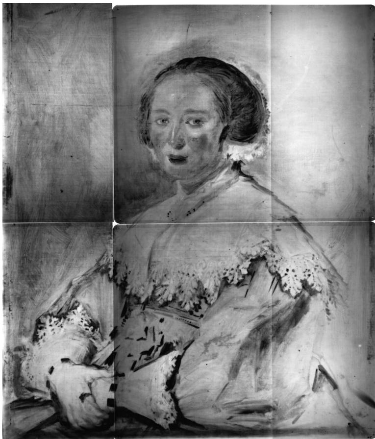
Fig. 3.11 Neutron-Autoradiograph of Fig. 3.1 (fifth recording)
