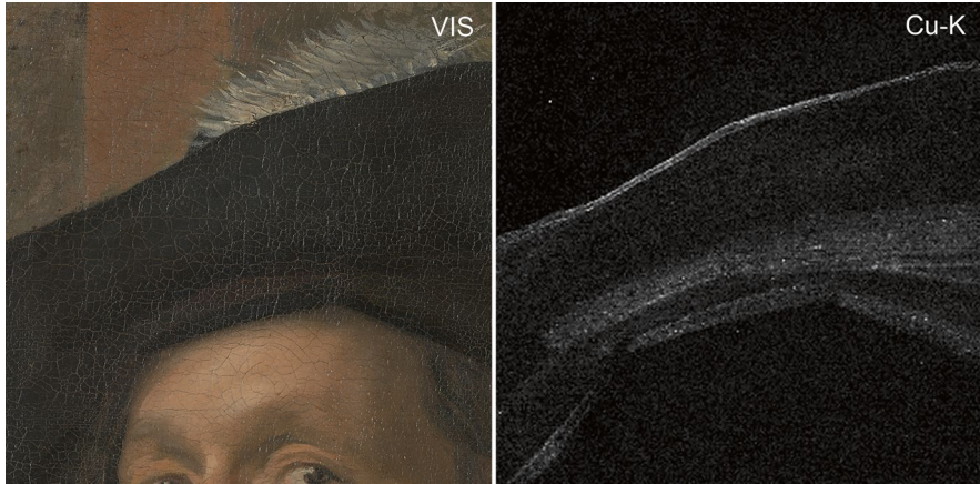
Detail of Fig. 6.5: visible light image and copper (Cu-K) map, in 'sync mode' ( sn.pub/qx5k1z )
