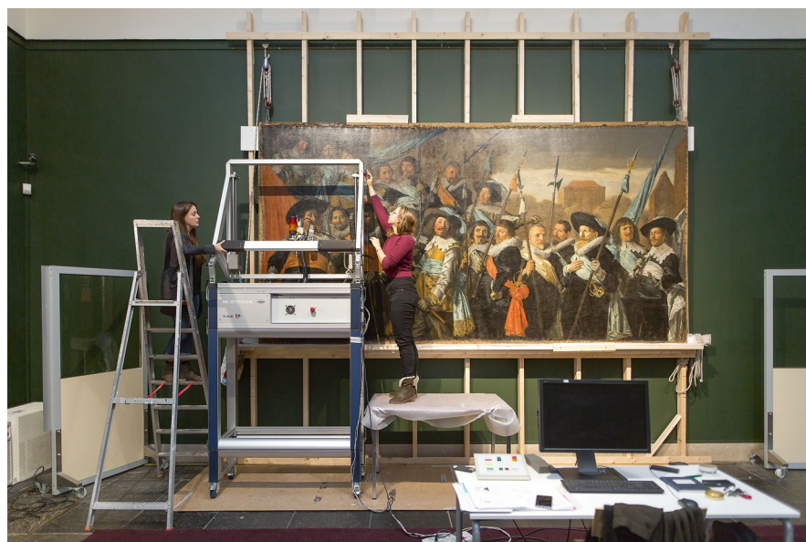
Fig. 6.8 MA-XRF scanning at the Frans Hals Museum by Nouchka De Keyser and Jennie Allred, Oct 2017
