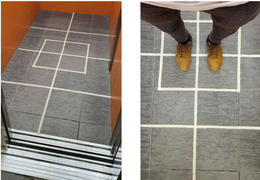
Fig. 10.5 Performing the ground-truth study to validate the analysis model and SES-PS: sections of the location analysis model marked down on the elevator floor with paint tape (left), and the test passenger carrying out the experiments standing in Section 9 in the middle of the elevator cabin, facing the doors (right)
