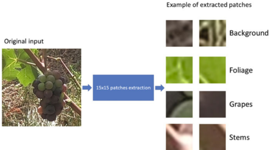
Fig. 9.2 Examples of pixel neighborhoods extracted from a vine image (Pinot Noir, during veraison) (Mohimont et al. 2022)
