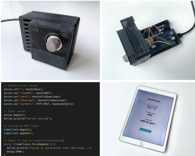
Fig. 6. Parts of the System Prototype for Monitoring CO 2 Emission Levels.
