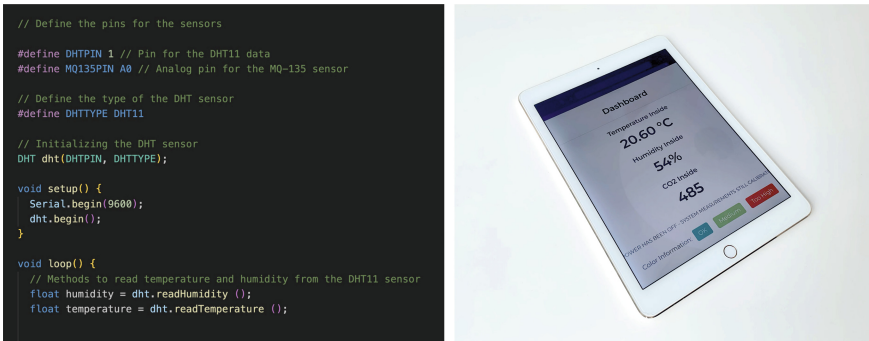
Fig. 3. Arduino code and visualization dashboard coded with HTML, CSS, and JavaScript.
