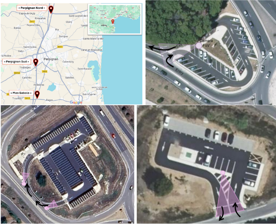
Fig. 1. Map view (upper left) and aerial views of the carpooling carparks: Perpignan Nord (upper left), Perpignan Sud (lower left) and Mas Sabote (lower right). Purple cones represent the cameras' lines of sight. (Color figure online)
