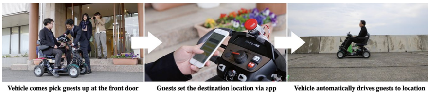
Fig. 6.2 Basic flow of the mobility service. An autonomous personal mobility vehicle will come pick guests up and drive them to their destination on their own
