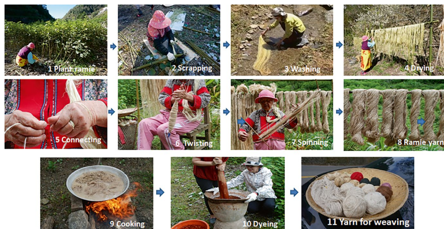
Fig. 9.4 Turning ramie into yarn requires a complex process of more than ten steps. It takes about 1 month of work to make 1 kg of ramie yarn that can be used for weaving. (Photos taken by authors in 2020)
