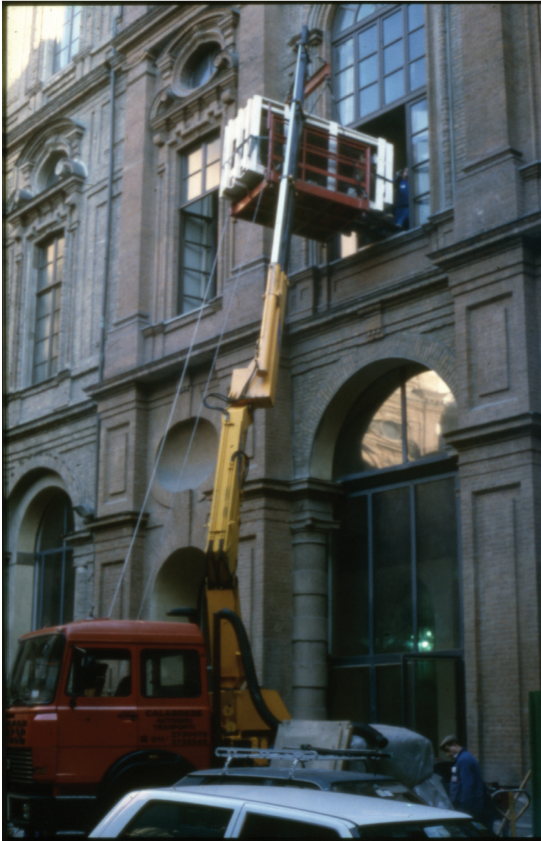
Figure 4.6 Giuseppe Penone's Albero Porta – Cedro had to be lifted into the galleries through an open window due to its size and weight, as shown in this photograph. Courtesy of the Museo Egizio, photo by Andrea Di Dio.
