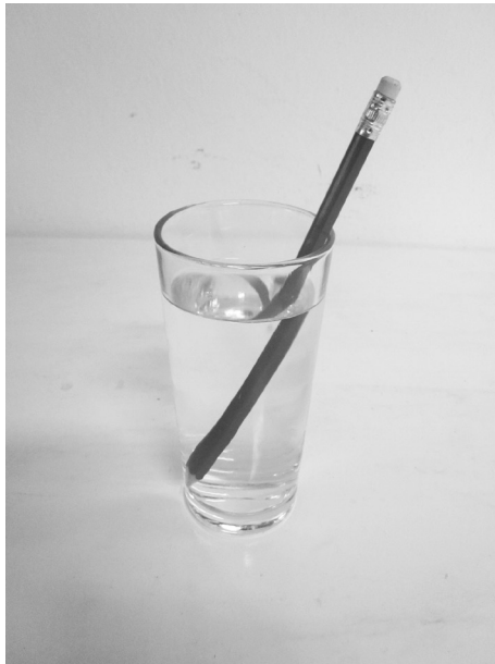
Figure 1.2 Refraction in a glass of water (Source: Meganbeckett27, Wikimedia Commons, CC BY-SA3.0)
