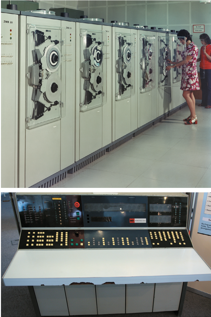
Figure 3: Magnetic tape units (top) and control panel (bottom) of the R 300.
